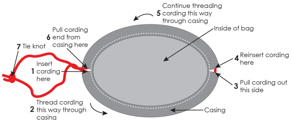
**Step 10:** Insert the remaining cording piece into the casing on the right edge of the bag. Thread through as you did in Step 9. Each casing will now have two pieces of cording running through it. Tie a knot as you did in Step 9.
